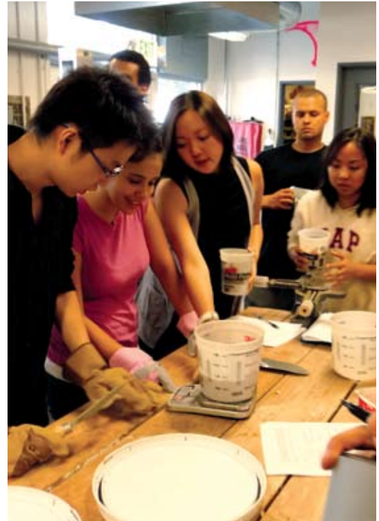
Built to Last: Architecture students prepare concrete cylinders of various strengths to test their structural integrity.
